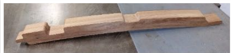
Panel post machined using jig
