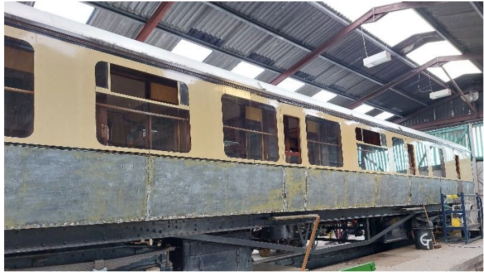
6705 with panels stripped ready for painting
