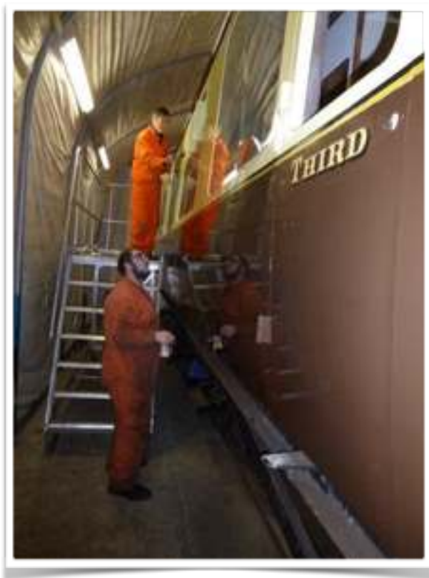
This picture was taken on 5th November showing the coach being varnished by Duncan Hensley and Chris Walters. It is lettered and lined out, using the exact livery she carried when she rolled out from Swindon works in 1938.
