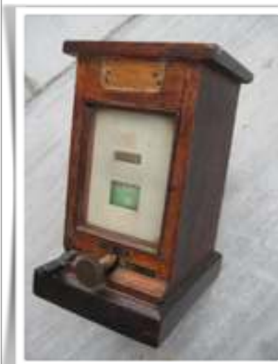
A standard GW lamp case with pyrometer in the lid and burner interior alongside, and a signalbox lamp repeater
